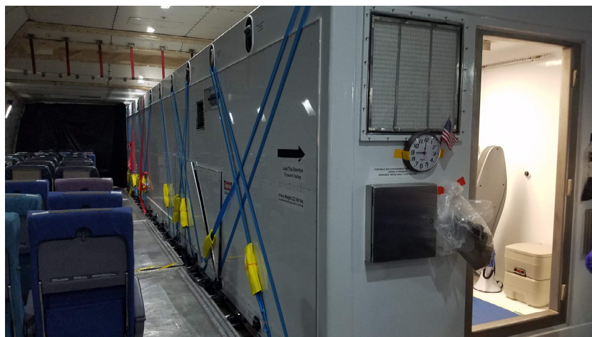
Figure 1. Containerized Bio-Containment System.
