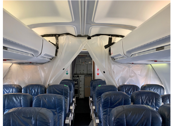
Figure 2. Isolation Zone Shroud.
